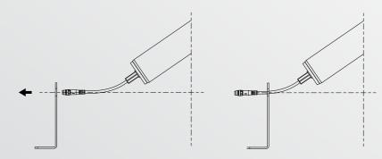
2. Align the other side of the motor with the opening in the frame on the opposite side.
