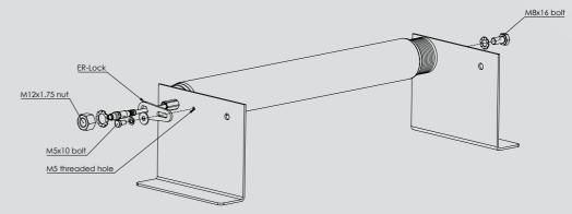
1. Press the HEX shaft inwards and place the E-roller between the two frames. When correctly aligned, the HEX shaft will lock itself inside the fame.
