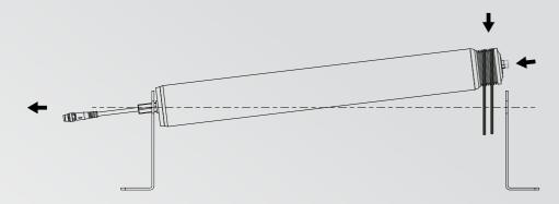
Note: when installing an E-roller with tapered elements (i.e. in a curved section), the attachment shaft will be positioned under a small angle. To prevent damaging the motor, a suitable angle compensator must be used for mounting the E-roller. This is not included in the default scope of delivery.
