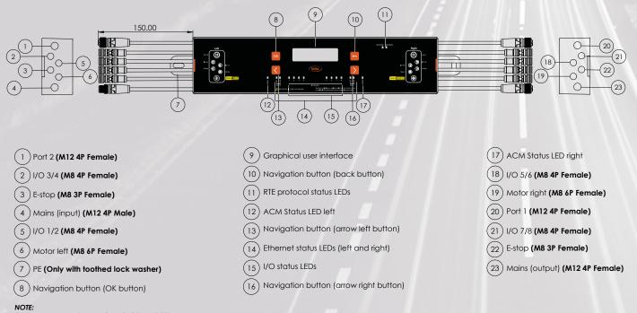
The power connectors are **S-coded** (4 and 23) The ethernet connectors are **D-coded** (1 and 20) The remaining connectors are **A-coded** The backplate is anodized, PE connection only guaranteed when using the supplied toothed lock washers
